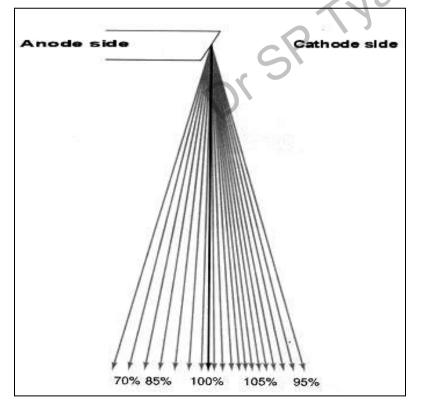
This is because of the fact that the x-rays are emitted from target in all the directions and those emerging parallel to the angled target is attenuated by target itself. Thus the intensity of x-ray on anode side is low. This difference in intensity may be as high as 40%.
